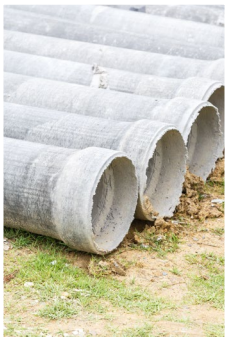
Asbestos Cement (AC)
