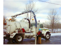
High velocity cleaner with vacuum device to remove grit & debris
