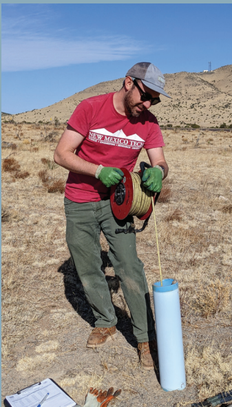
Measuring the depth to water in a well near Magdalena.
